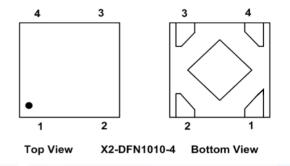
PIN1-Vout, PIN2-GND, PIN3-EN, PIN4-VIN
