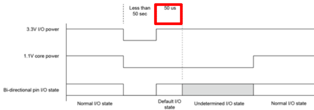
Figure Error! No text of specified style in document.-9 Timing Sequence with Undetermined I/O State
