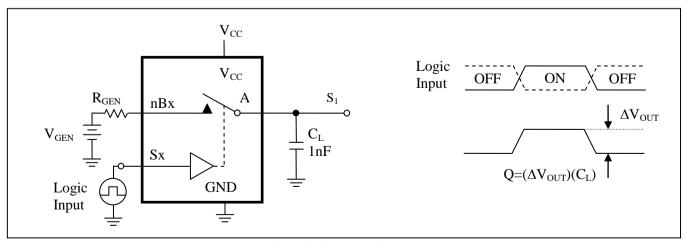
Figure 3. Charge Injection Test
