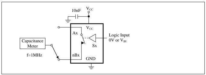
Figure 6. Channel Off Capacitance
