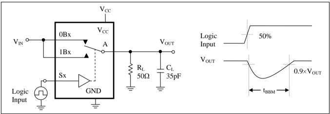
Figure 2. Break Before Make Interval Timing
