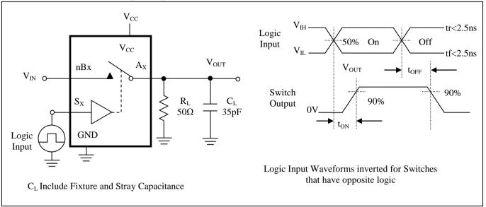
Figure 1. Turn ON/OFF Timing
