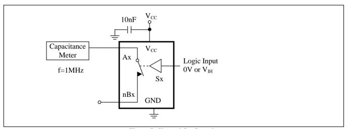
Figure 7. Channel On Capacitance
