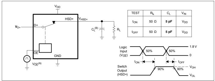
Figure 1. Turn-On (t<sub>ON</sub>) and Turn-Off Time (t<sub>OFF</sub>)
