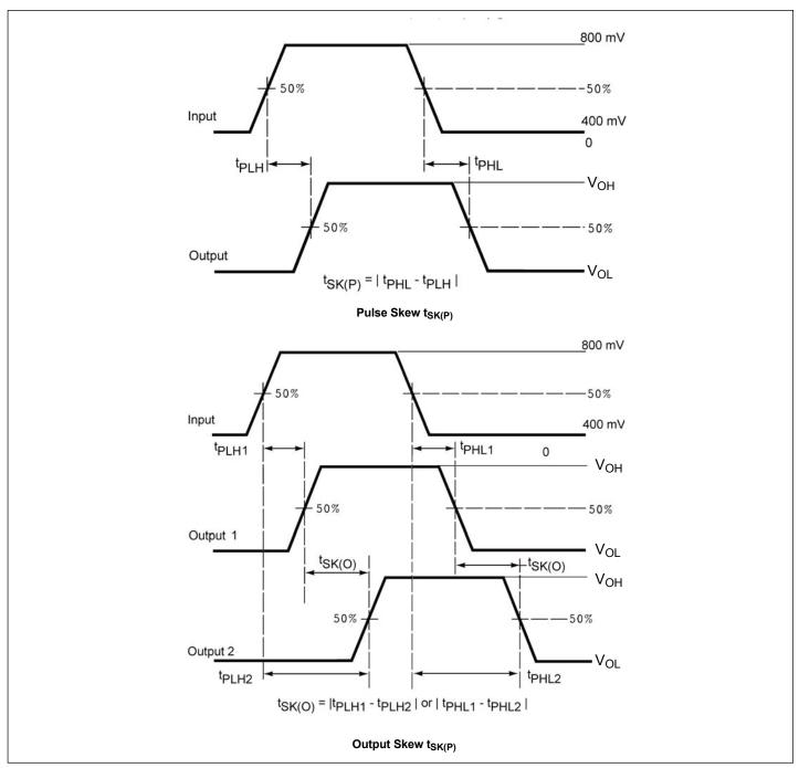
**Figure 5. Skew Test**
