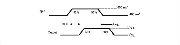
**Figure 4. Propagation Delay**
