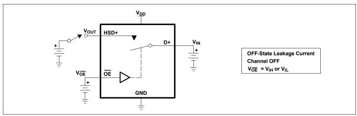
Figure 7. OFF-State Leakage Current
