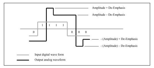
Figure 5-1 Driver Output Waveform
