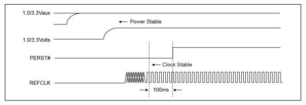
Figure 11-1 Initial Power-Up Sequence
