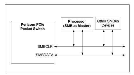
Figure 6-1 SMBus Architecture Implementation on PI7C9X2G404EL
