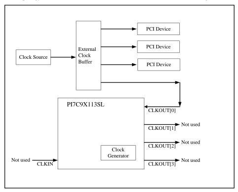
In this configuration, user simply connects the external clock from the clock buffers to CLKOUT0. And user needs to make sure the clock is preset (toggling) before the fundamental reset de-asserted (e.g. PERST\_L deassertion).
