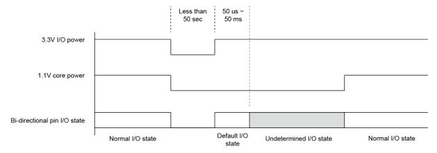
Figure 14-1 Timing Sequence with Undetermined I/O State
