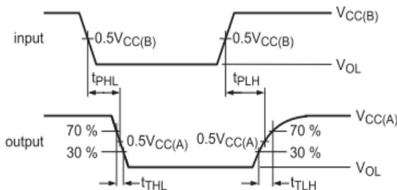
Figure 5: Propagation Delay and Transition Times B→A
