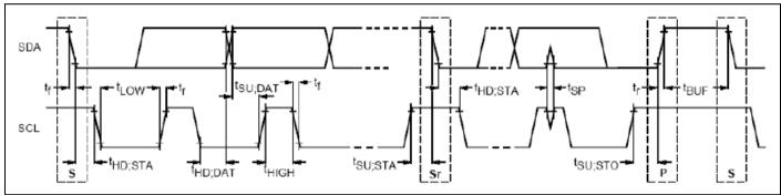
Figure 3. Definition of Timing for Full-Speed Mode Devices on the I<sup>2</sup>C Bus
