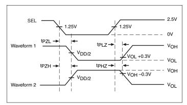
**Voltage Waveforms Enable and Disable Times**
