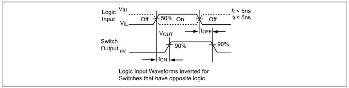
Figure 2. AC Waveforms
