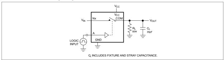
Figure 1. AC Test Circuit
