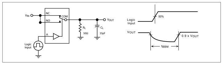
Figure 3. Break Before Make Interval Timing
