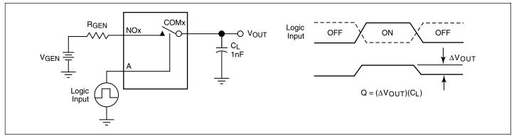
Figure 4. Charge Injection Test
