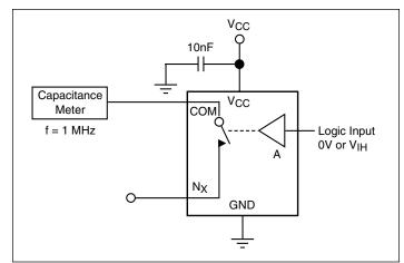
Figure 8. Channel On Capacitance
