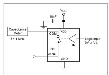
Figure 8. Channel On Capacitance
