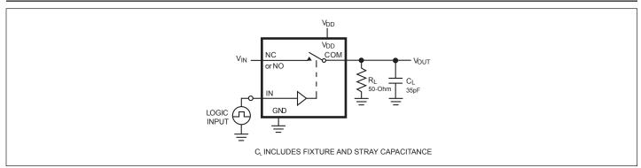
Figure 1. AC Test Circuit
