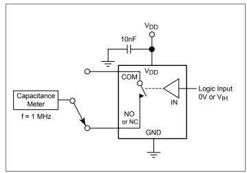
Figure 7. Channel Off Capacitance
