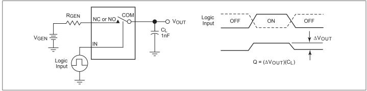
Figure 4. Charge Injection Test
