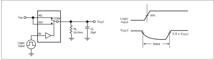
Figure 3. Break Before Make Interval Timing
