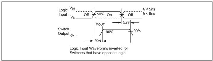
Figure 2. AC Waveforms
