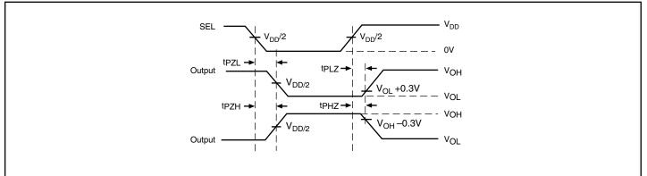
Voltage Waveforms Enable and Disable Times
