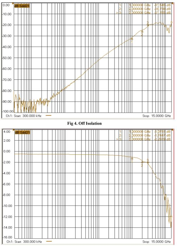
Fig 5. Insertion Loss
