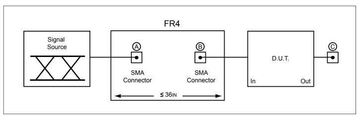
**Test Condition Referenced in the Electrical Characteristic Table**
