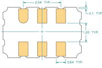
\*Extended high frequency power decoupling is recommended (see test circuit for minimum recommendation). To ensure optimal performance, do not route RF traces beneath the package.
