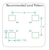
\*Extended high frequency power decoupling is recommended (see test circuit for minimum recommendation). To ensure optimal performance, do not route RF traces beneath the package.
