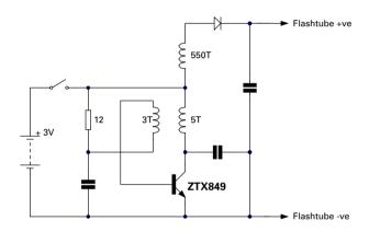
Component size and capacitor re-charge times are a major consideration for camera flashguns. Regular TO220, TO126 or SM D-PAK packaged chips, although bigger, cannot match the performance of the E-Line (TO92 style) Matrix Bipolar chip family. Zetex transistors exhibit lower saturation voltages, higher h<sub>FE</sub>, a higher current gain hold-up/silicon area, and a more efficient switching performance than any of the devices available from the aforementioned packages.
