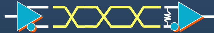
Serial Differential Interface: (1Gb / 10Gb Ethernet, USB, PCI Express, HDMI, DisplayPort, Fiber Channel, SAS, SATA...)
