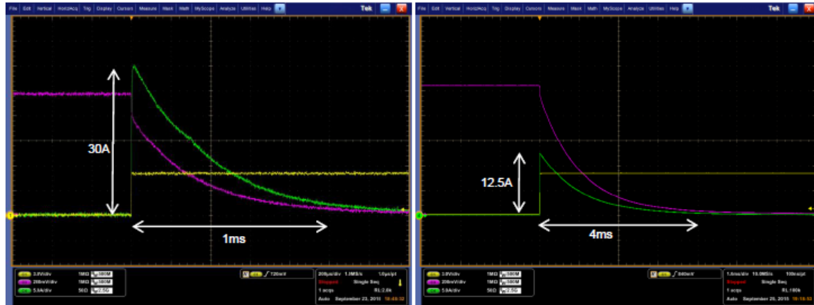
Figure 3. Results recorded without (left) and with (right) 50mΩ series discharge resistor.
