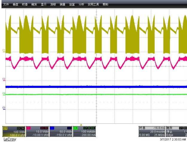
LED Open Protection (V in =120V AC , Y-V DRAIN , R-V CC , B-V out , G-I LED )
