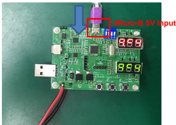
Figure 7: The Test Tool Input & Output Location
