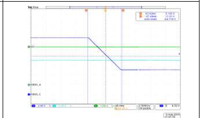
Input: 115V AC / 60Hz, Output: 12V to 5V Transition Time: 90.42ms
