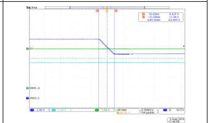
Input: 115V AC / 60Hz, Output: 12V to 9V Transition Time: 40.42ms
