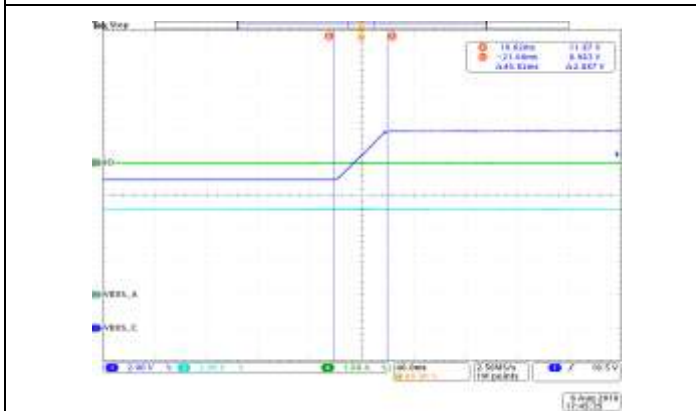
Input: 115V AC / 60Hz, Output: 9V to 12V Transition Time: 40.82ms
